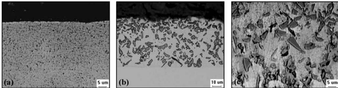
Figure 1 Metallograph of the cross-section of (a) Ni-P-PTFE and (b) Ni-P-SiC (c) Ni-P-PTFE-SiC.
