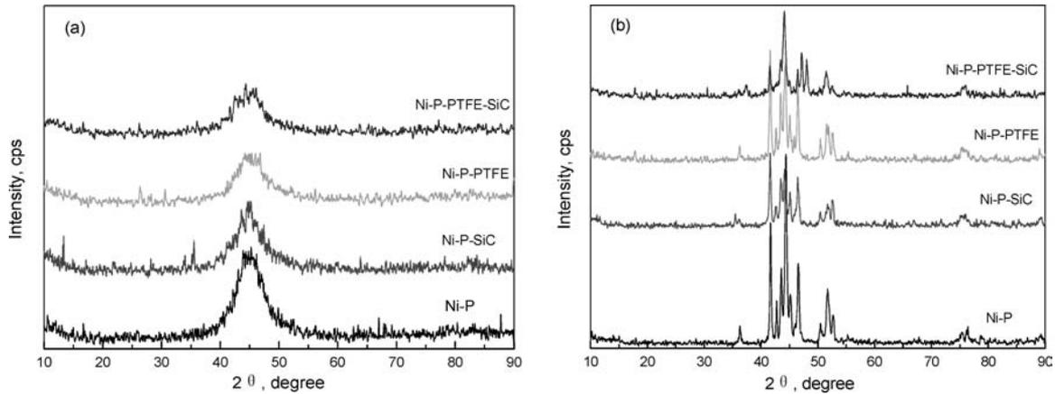
Figure 3 XRD patterns of (a) as-deposited and (b) heat-treated at 400 °C for 1 hr of Ni-P and Ni-P composites.
