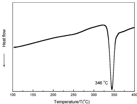
Figure 2 DSC thermogram of the Ni-P-PTFE-SiC at a heating rate of 20 °C/min.
