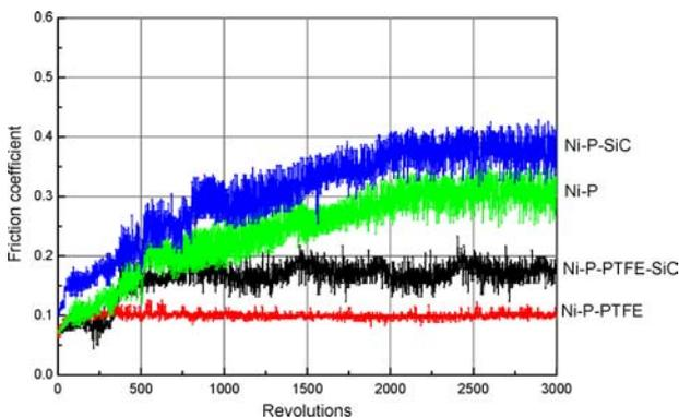
Figure 5 Friction coefficient vs. revolutions for Ni-P and Ni-P composite coatings.
