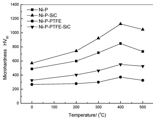
Figure 4 The microhardness of Ni-P and Ni-P composite coatings (at as-deposited, 200 °C, 300 °C, 400 °C, 500 °C for 1 hr, respectively).
